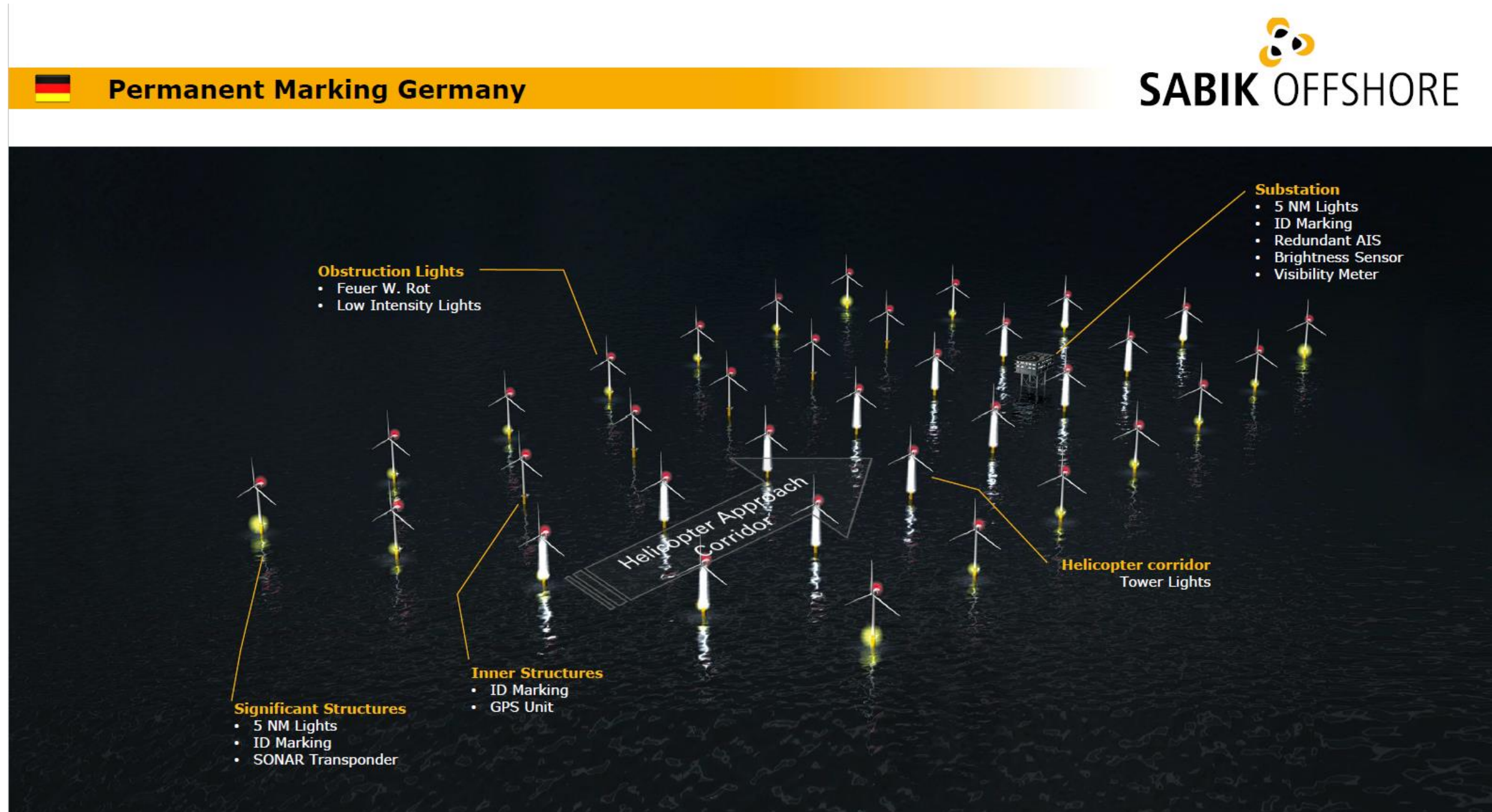
Fig. 2: German operational-phase marking and lighting scheme (Source: Sabik Offshore)
