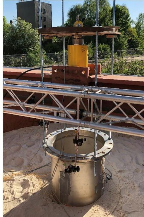
Fig. 4: static load test to determine the breakout resistance
