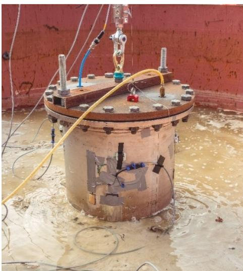
Fig. 3 pile extraction with over pressure
