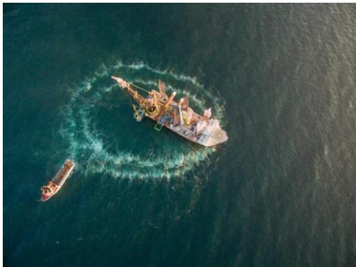
Fig. 1: Double Bubble Curtain noise mitigation system (photo © Vattenfall)
