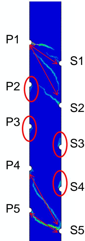
Max. principal plastic strain in the grout at ULS compressive load ( $F_{ULS} = 7.55$  MN)
