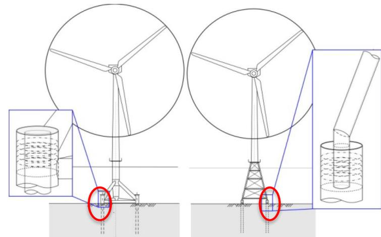
OWT with a tripod / jacket substructure and detail of a grouted joint (Schaumann et al., 2013)
