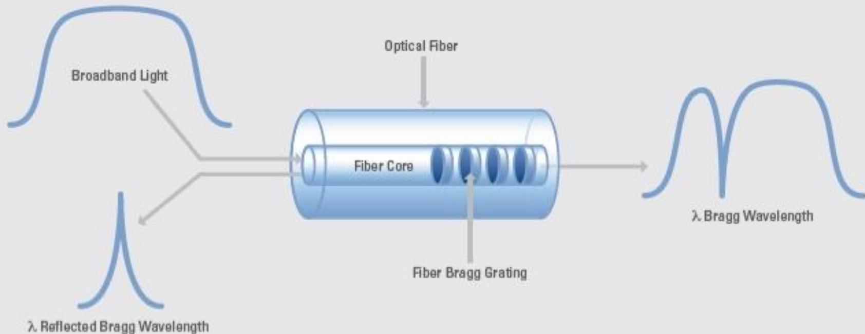
FBG advantages: robust (harsh conditions), immune to electromagnetic interferences, multiplexing ...
