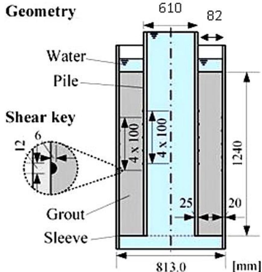
Cut-off view of a grouted connection specimen (tripod structure in a scale of 1:4)
