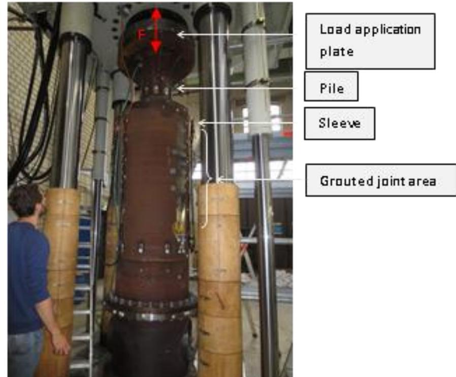
Grouted connection specimen in the servo-hydraulic testing machine
