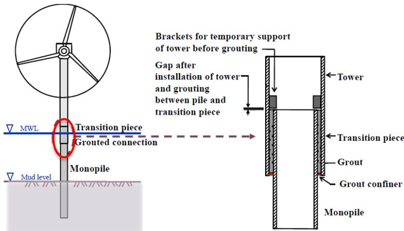
OWT with a monopile substructure and detail of a grouted joint (DNV, 2014)
