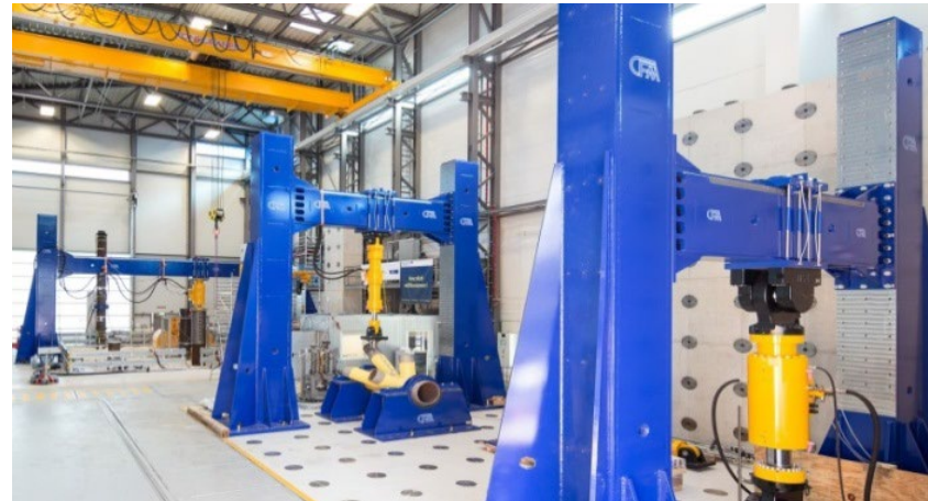
Strong floor: Horizontal 18,5 x 9,5 m (L x B); Vertical: 9,5 x 10 x 8 m (L x B x h)
