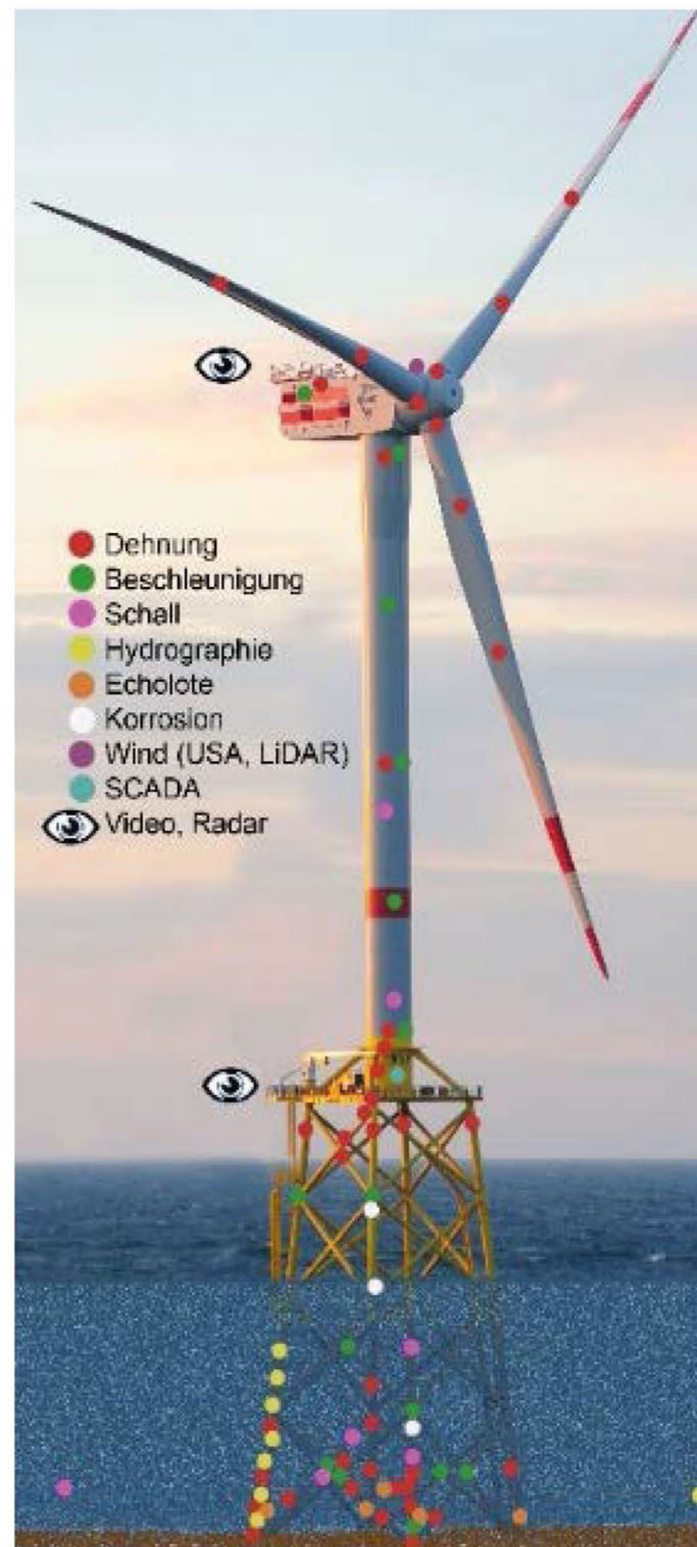
Measurement sensors at two wind turbines in alpha ventus © 2020 Fraunhofer IWES
