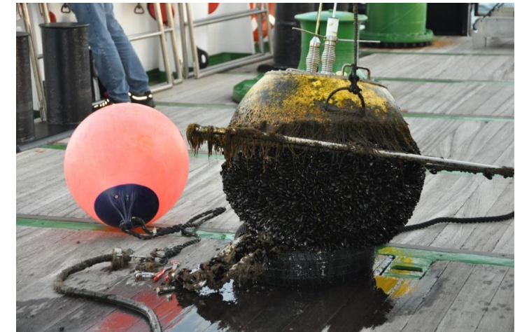
DWR buoy after recovery
